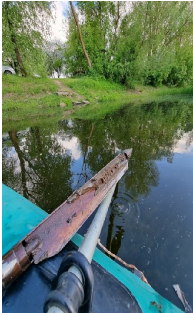
Figure 106. Measuring thickness of accumulated sludge (Photo: A. Balevičius)
